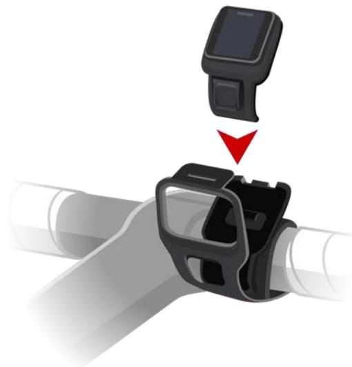
5. Close the handlebar strap over the top of the watch, attaching it to the top of the holder using the clip.
