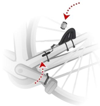
Once you have adjusted the sensors to the right position, tighten the cable ties so they are held securely in place.
