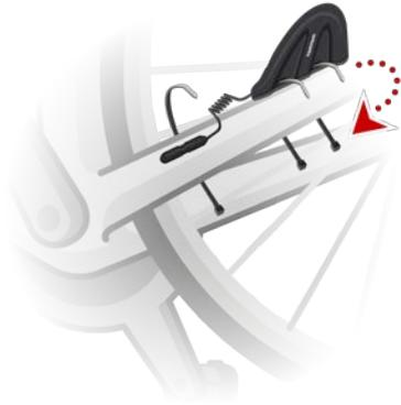
2. Attach the spoke magnet to one of the spokes on your bike. The magnet should face the chainstay where you attached the chainstay sensor.
