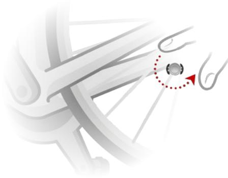
3. Adjust the position of the spoke magnet and the chainstay sensor so that when the wheel turns the spoke magnet passes the tip of the main body of the chainstay sensor.
