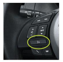
Voice recognition for infotainment is started using the push-to-talk button on the steering-wheel - this may depend on your car model.
