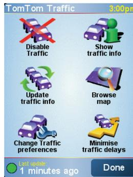
TomTom Traffic is a TomTom PLUS service that sends up-to-date traffic information to your NAVIGATOR. To use TomTom Traffic you must have a mobile phone with Bluetooth and a wireless data connection, for example, GPRS, EDGE, UMTS, CDMA.
