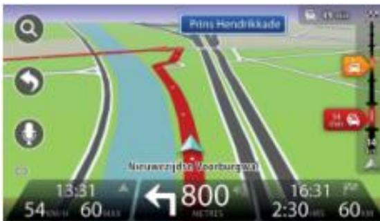
Go to the Main Menu from the Driving View. Push the stick right or up to focus on area (1). Push in the stick.
