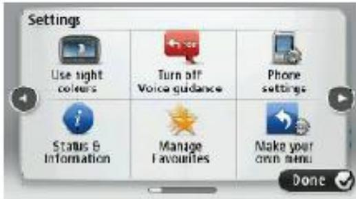
Move between menu buttons 1-6. Rotate the stick left or right.
