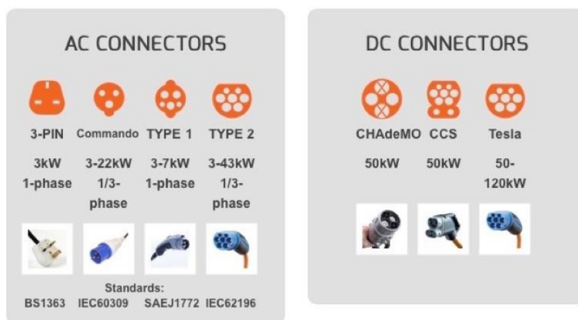
Fig. 8 Main types of electric vehicle connectors currently on the market
